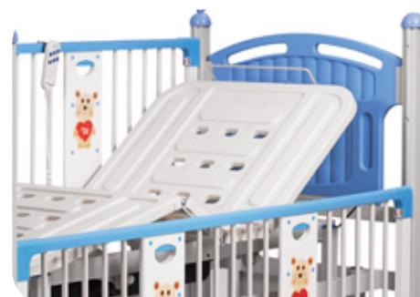
Suitable for cardiac massages. Made of 4 planes of injected polymers resting over a steel structure. Not having sharp edges, the rounded corners protect the crib operator. The central part is welded to the structure and The central part is welded to the structure and the rest are linked through steel bolts with specially rounded heads for a better finish.
